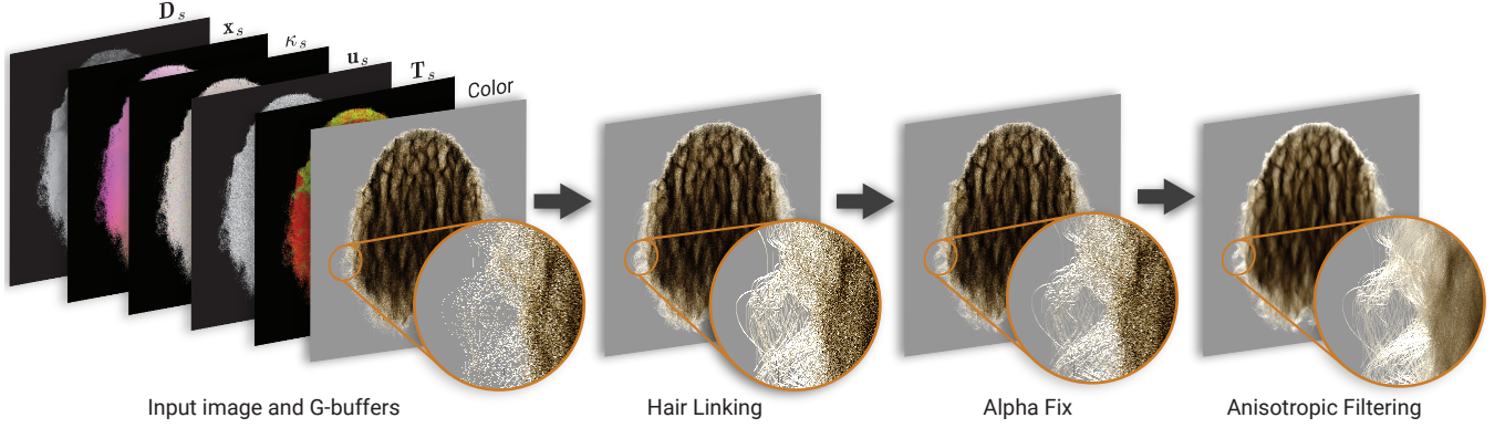
Figure 2: Overview of our hair linking and filtering pipeline. Starting from G-buffer data and a 1-spp input image, we first link disconnected flyaway fibers via a hair linking procedure. Next, an alpha fix step enforces energy conservation, mitigating transparency-induced artifacts. Finally, we apply anisotropic filtering to reduce noise while preserving high-frequency hair details.
