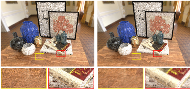
Figure 3: Impact of the ray differential structure in cache query and interpolation. Here, we compare the query results without (left) and with (right) the ray differential structure.
